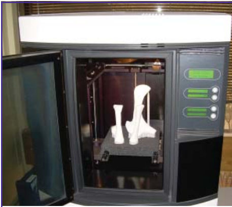
Newly completed bone models of juvenile sauropod bones ready to be removed from the 3-D printer.
